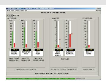
During transport of personell from shore to worksite or between worksites the motion trend displays can be used actively to reduce the motion discomfort that causes nausea and seasickness. This will make sure the personell arrives at site in good shape and ready to work.
